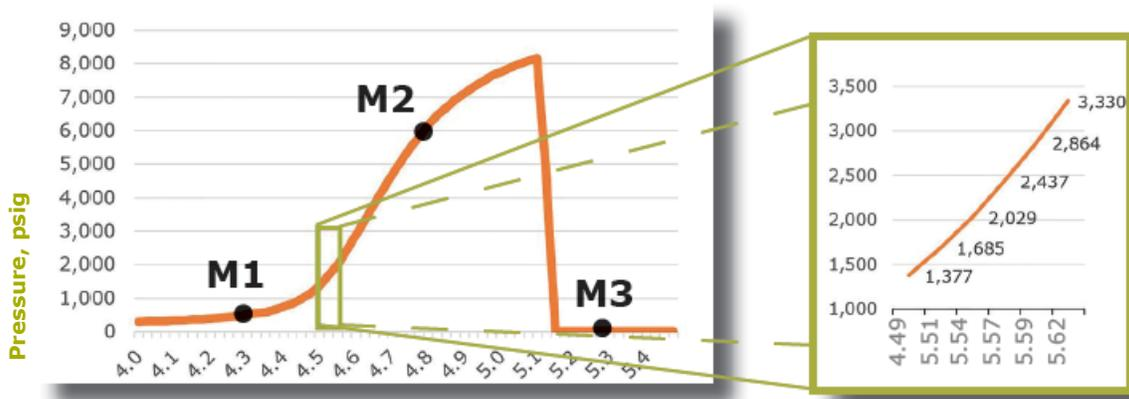
*This graphic illustrates how quickly pressure can spike, increasing 2,000 psig in 0.1 second. Typical data acquisition vans only measure 1-2 times per second, meaning the episode is unobserved (M1-M3), appearing as though the Well Casing Safety Plug activated low when it actually performed as calibrated.*
